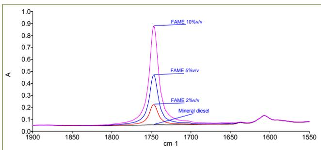
The Spectrum Two FT-IR provides fast and easy analysis of varying FAME concentrations in diesel fuel.
