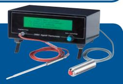
The Seta-Orbis Digistill D86 controller is a bench top unit designed for automated reading of atmospheric distillation data from a manual distillation instrument in accordance with ASTM D86 and equivalent methods.
